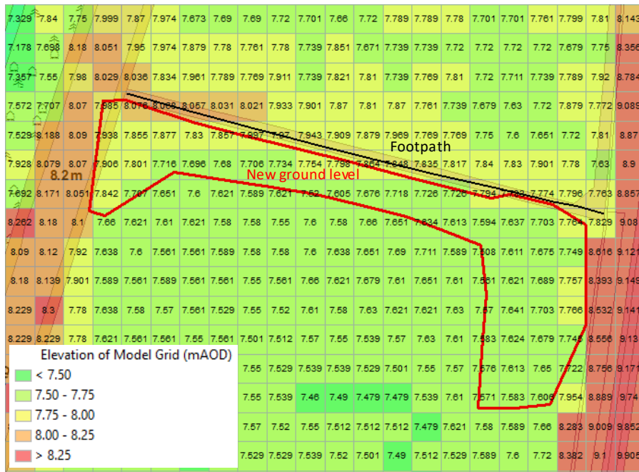
Figure 6-4: Updated model elevation grid Clange Road compound without vegetation and depression (red polygon) and with new footpath representation (black line)
